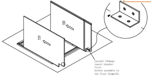
Step 3 : Install bottom panel. Insert the bottom panel (C) into groove of side panel(B) until it into the groove of front frame(A).
