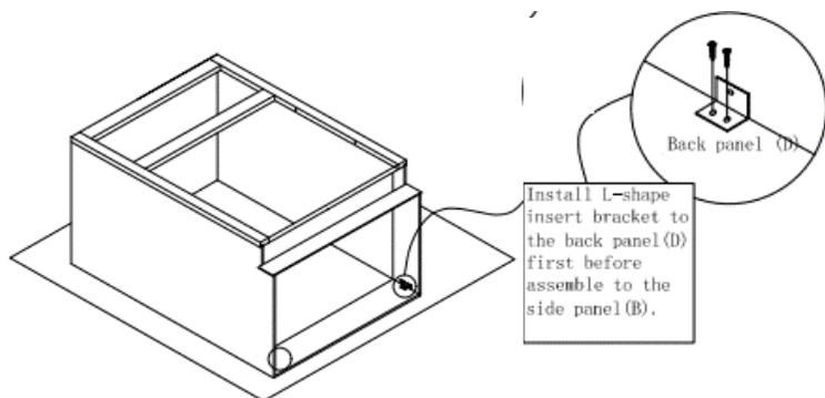
Step 8 : Install corner block. Install rainbow bracket to the side panel (B), front frame (A) and back panel (D) with the (5)  $\Phi 4 \times 16\text{mm}$  screw.
